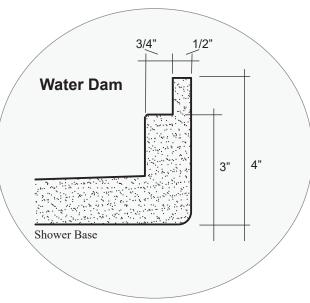
Water dam is provided on all sides of the base when using the independent raised threshold
